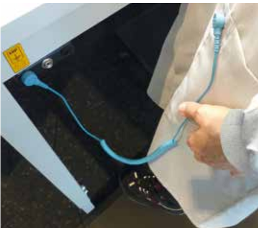
grounding via coilcord
