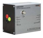
CISPR 15 edition 9 offers different methods for the measurement of radio disturbance characteristics of electrical lighting equipment. One of these is the CDNE method. This method specifies the use of a coupling/decoupling network for emission measurement (CDNE) to measure disturbance voltages in the 30 to 300 MHz frequency range. This method enables EUTs to be connected directly to the CDNE, allowing a single conducted emission measurement to replace a lengthy radiated emission test.
